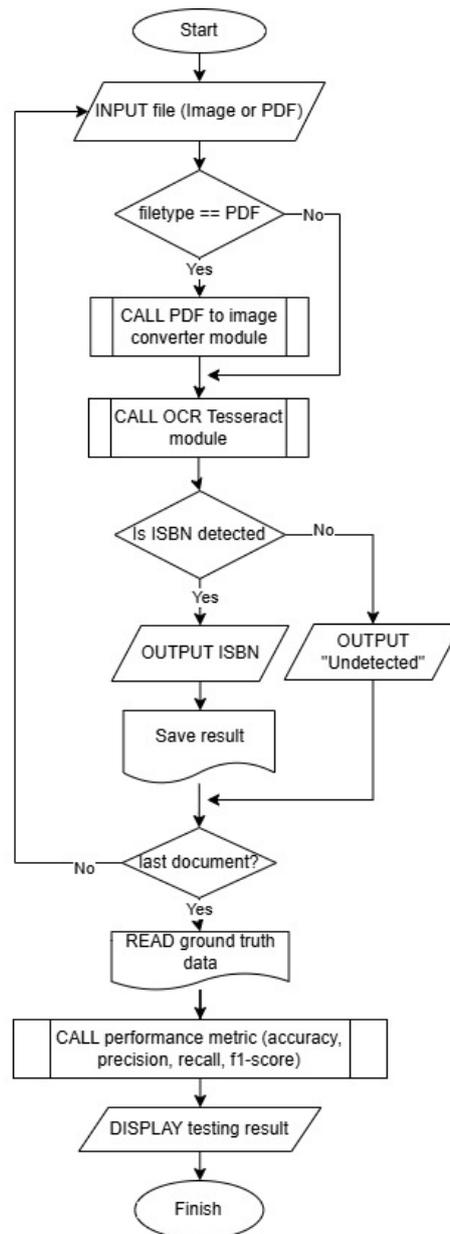
Figure 2. Flowchart of the OCR Process
