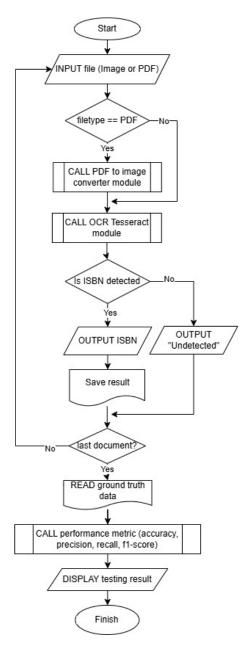
Figure 2. Flowchart of the OCR Process
