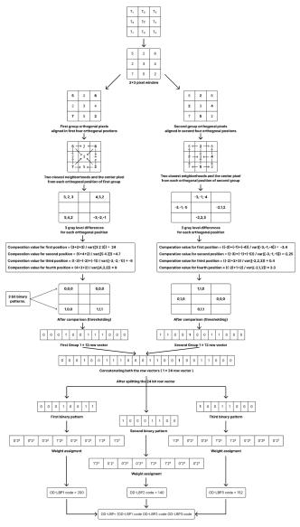
Figure 3. Demonstration OD-LBP process
