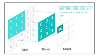
Figure 1. Convolution Process
