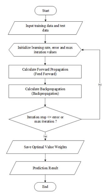
Figure 2. Backpropagation Method Flowchart
