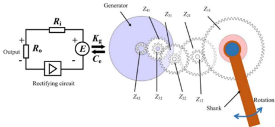
Figure 5. Schematic Diagram of Transmission on Energy Harvester
