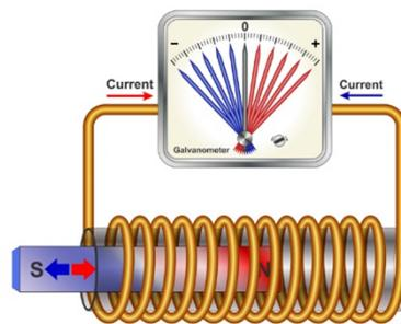
Figure 4. Electromagnetic Transducer
